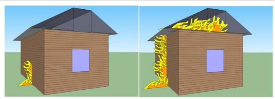
The most expensive school fires starts on the outside of the building, the fire spread up to the attic, where it spread quickly and can cause a total damage.
