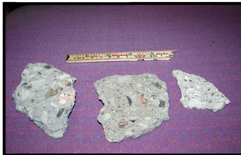
Figure 2.45 Flakes from spalling of normal strength SCC (left and middle flake) and high strength SCC >100MPa during fire testing, (right flake). The thickness of the spall from the high strength SCC is only a few millimetres. Photo Robert Jansson.
