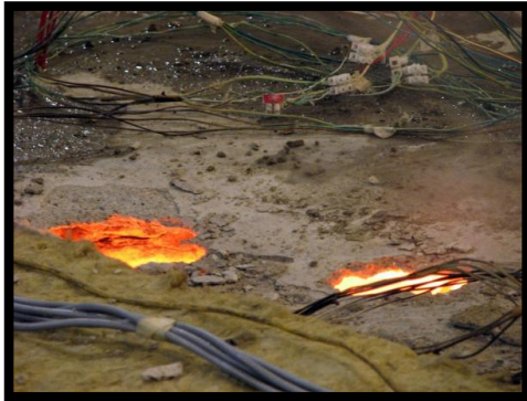
Figure 2.29 Severe spalling breaking through the 200 mm thick concrete specimen after 40 minutes of exposure to the hydrocarbon fire curve. Photo Robert Jansson
