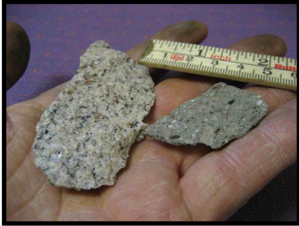
Figure 2.46 Flakes from spalling of granite and high strength SCC (> 100 MPa during fire testing). They exhibit a similar thickness of about 5 millimetres. Photo Robert Jansson.
