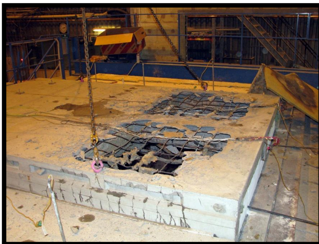
Figure 2.30 Severe fire spalling during fire testing of a high strength concrete floor slab exposed to unilateral fire. Photo Robert Jansson (published with permission of the client).
