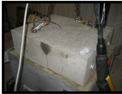
Figure 2.36 One sided heating of small specimens from the underside. (Left) Small slab loaded in compression, example of crack evolution in the load direction. Water is pouring out from the horizontal crack. (Right) Unloaded small slab, cracks develop vertically from the heated surface.
