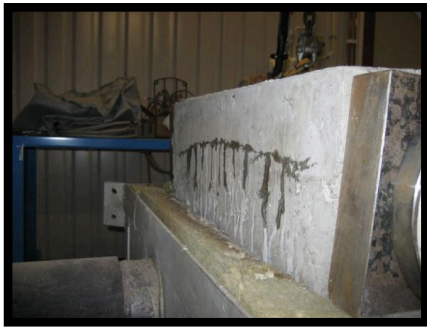
Figure 2.36 One sided heating of small specimens from the underside. (Left) Small slab loaded in compression, example of crack evolution in the load direction. Water is pouring out from the horizontal crack. (Right) Unloaded small slab, cracks develop vertically from the heated surface.
