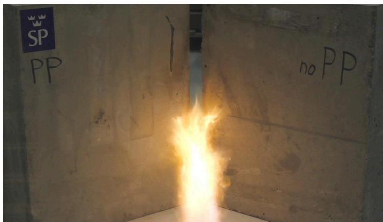
Figure 2.33 First heating of the corners of the specimens, no spalling recorded (Jansson and Boström, 2012).
