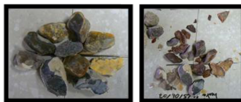
Figure 2.3 Flint before and after heating. The aggregate splits violently as observed by Mindeguia (2009).
