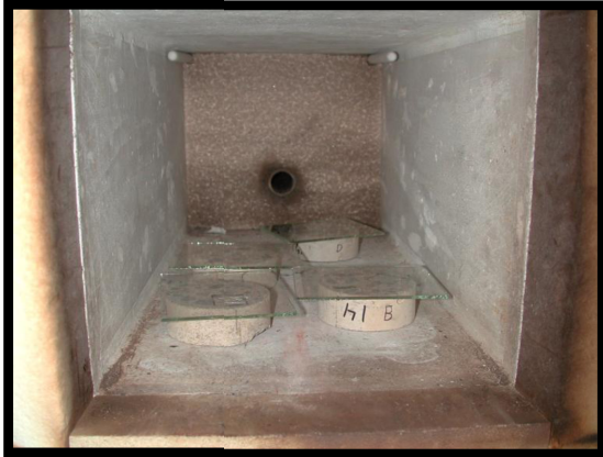
Figure 4.5 Test specimens in oven with PP fibres between the concrete and the glass. Photo: Robert Jansson
