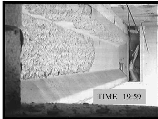
Figure 2.39 Loaded pre-stressed beam tested during the I-beam tests with ISO 834:1977 fire exposure. The cover of the web from the middle to the \frac{1}{4} point of the beam has spalled away.
