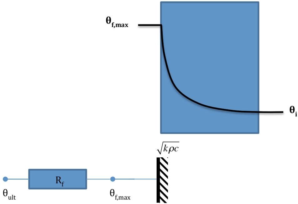
Figure 10 Temperature distribution within a semi-infinite surrounding structure with the approximation  $\theta_f = \theta_s$ . The series below shows an electrical analogy with the resistances and the temperatures across the surrounding structures after long time at steady state.
