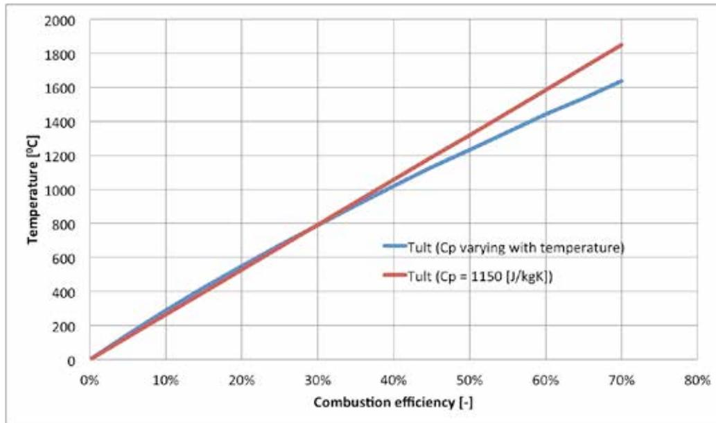
Figure 7 The ultimate temperature as a function of combustion efficiency with the specific heat capacity,  $c_p$  either depending on temperature or assumed constant.
