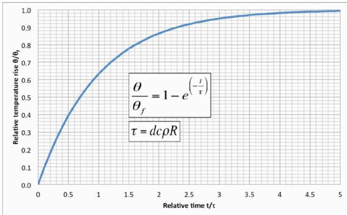
Figure 19 General solutions for both equation (46) and (47) with relative temperature rise and relative time.
