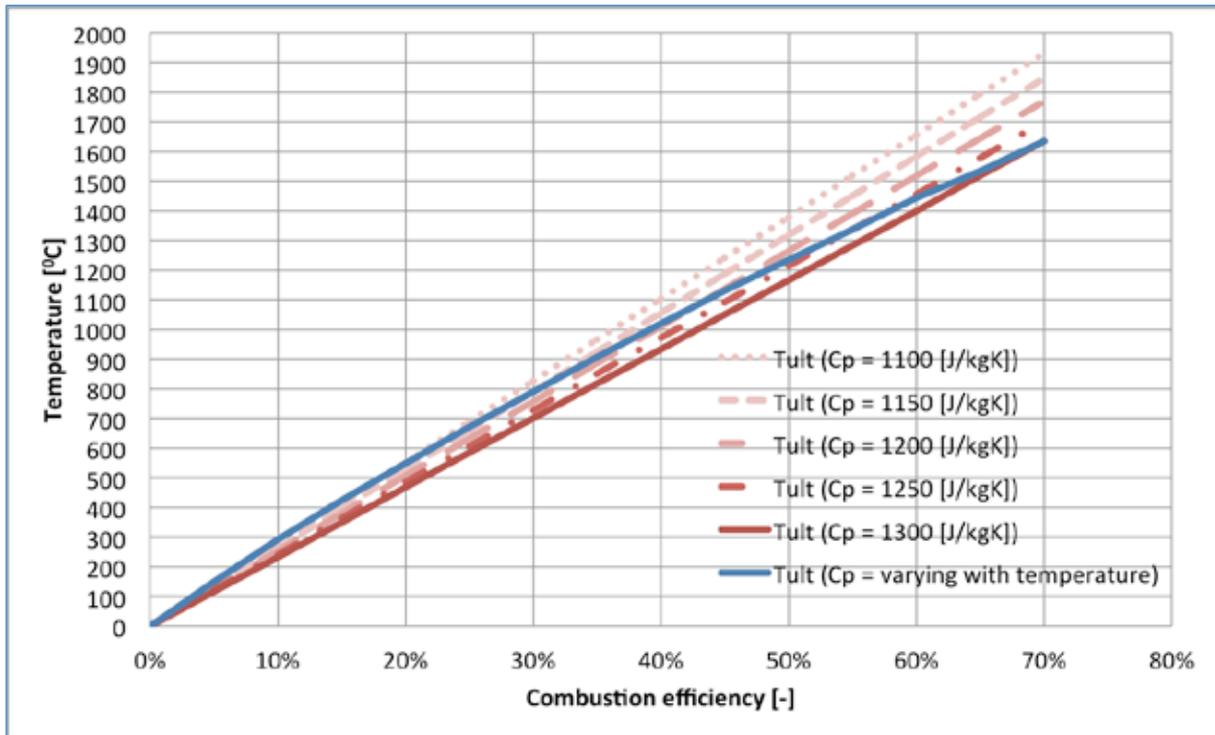
Figure 23 Impact on the ultimate fire temperature if the specific heat capacity of air is chosen as a constant value or as a function of temperature.
