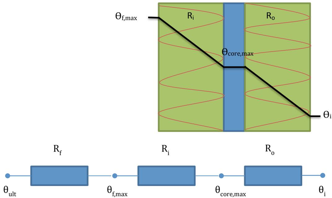
Figure 13 Temperature distribution within a thermally thin structure with insulation. The series below shows an electrical analogy with the resistances, heat capacity of the core and the temperatures across the wall. The heat transfer resistances between the air and the surrounding structures are included in  $R_i$  and  $R_o$ .
