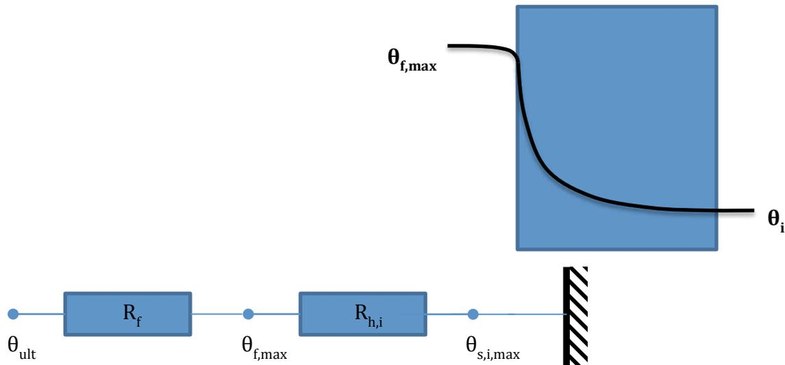
Figure 9 Temperature distribution within a semi-infinite surrounding structure. The series below shows an electrical analogy with the resistances and the temperatures across the surrounding structures after long time at steady state.
