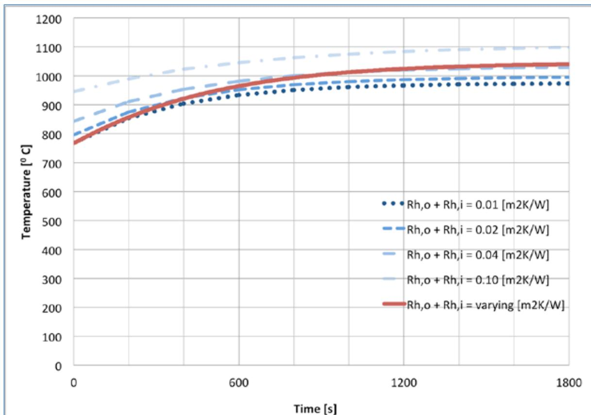
Figure 26 Fire temperature with constant- and varying convection and radiation heat transfer resistances.  $R_{ins,i} = R_{ins,o} = 0.052 \text{ m}^2\text{K/W}$ .  $R_{h,i}$  and  $R_{h,o}$  are varying as in equation (67) and (68).
