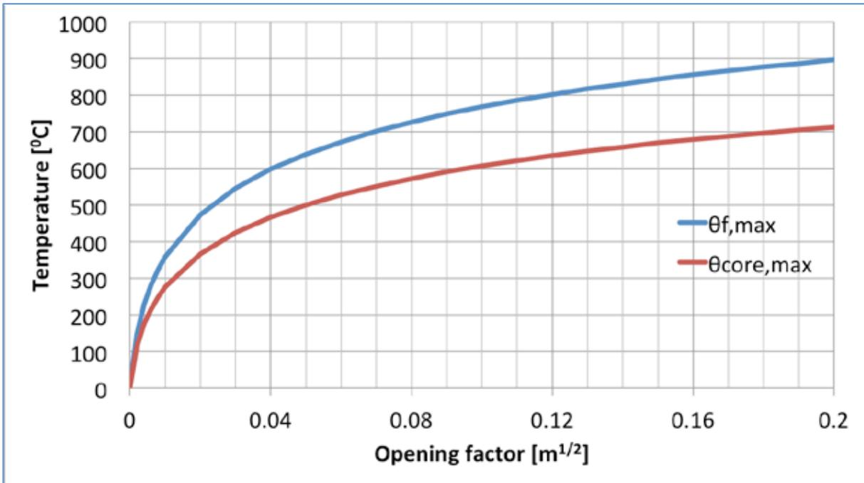
Figure 12 Maximal fire- and core temperature rise for a compartment with thermally thin surrounding structure for different opening factors. The heat transfer coefficients  $h_{c,i} = 25 \text{ W/m}^2\text{K}$ ,  $h_{c,o} = 4 \text{ W/m}^2\text{K}$ ,  $c_p = 1150 \text{ J/kgK}$ ,  $\varepsilon = 0.8$ . The thermal resistances  $R_{h,i}$  and  $R_{h,o}$  has been calculated as a function of temperature, described in chapter 4.6.
