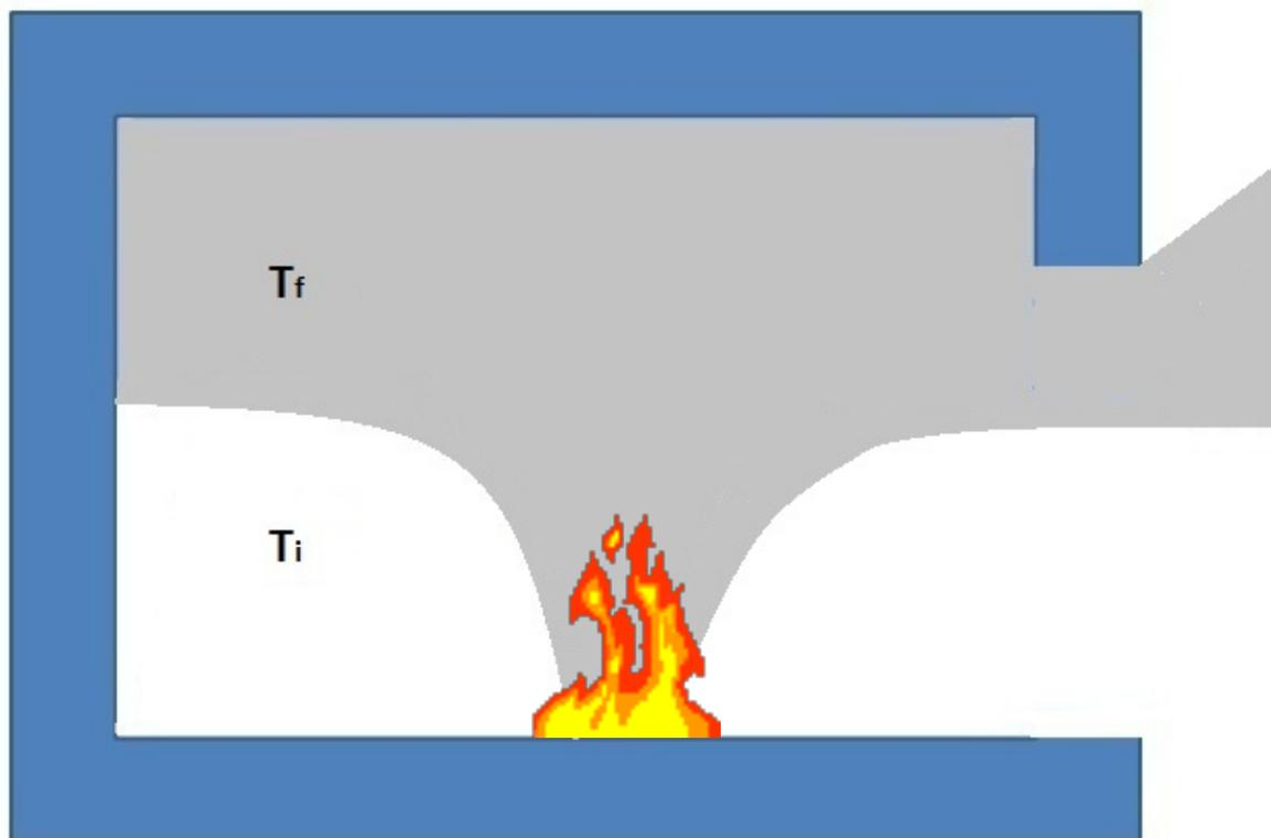
Figure 4 Illustration of two-zone model.
