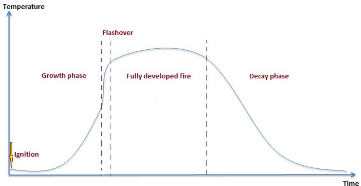
Figure 1 Schematic illustration of fire development.
