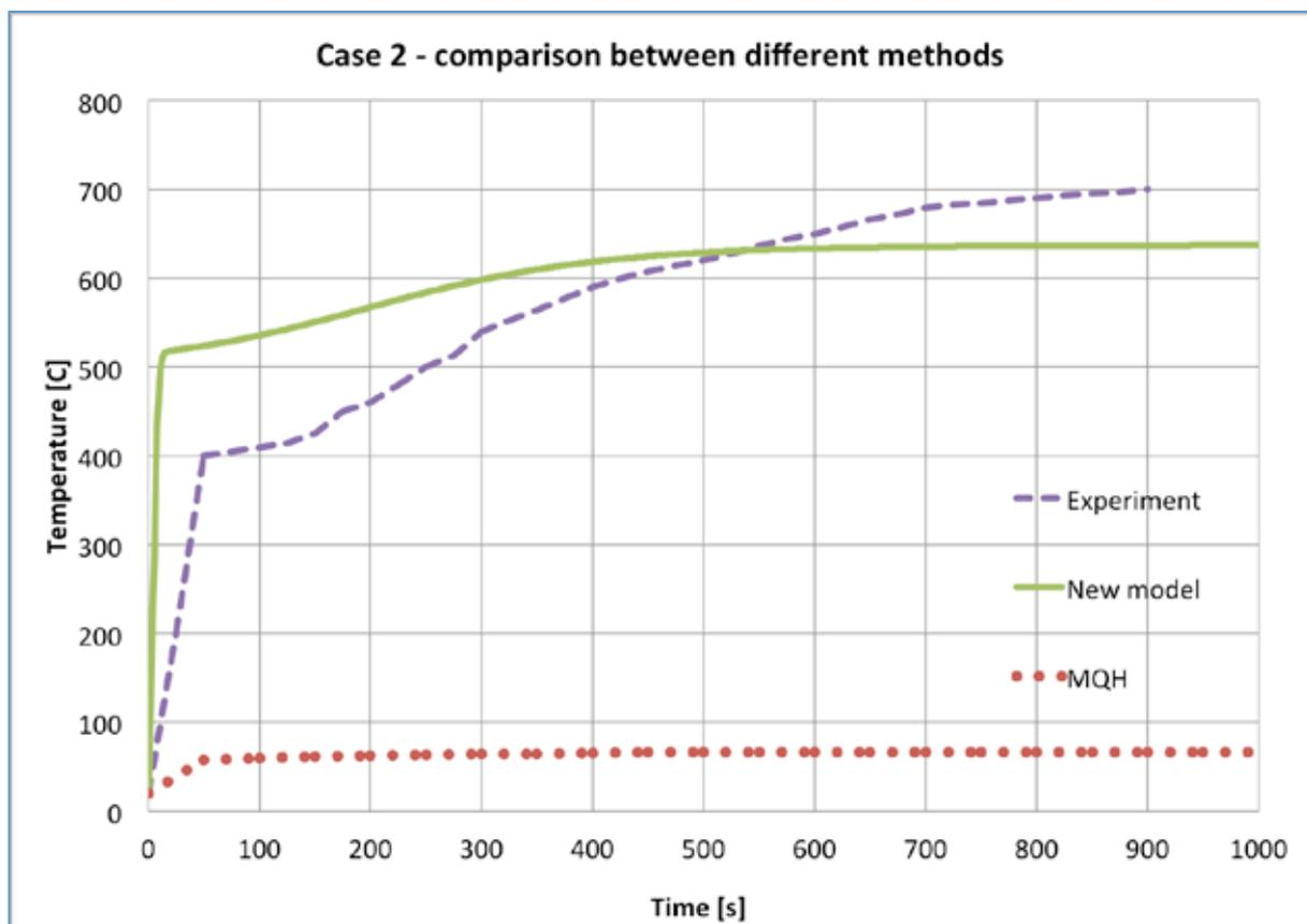
Figure 33 Comparison between different calculation methods for a steel container without insulation (case 2) and the experimental result (Back 2012).
