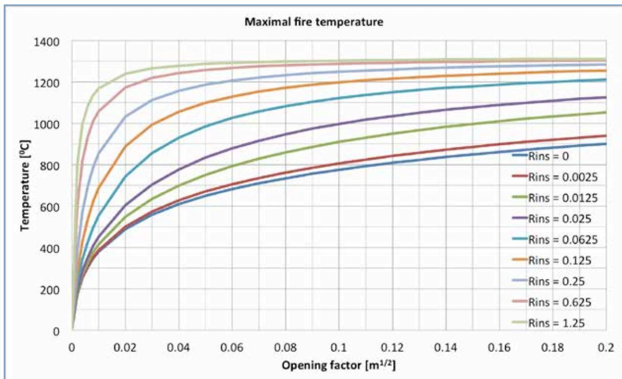
Figure 15 Maximal fire temperature rises for insulated thermally thin surrounding structure with different amount of insulation. The heat transfer coefficients are  $h_{c,i} = 25 \text{ W/m}^2\text{K}$  and  $h_{c,o} = 4 \text{ W/m}^2\text{K}$  and the specific heat is  $c_p = 1150 \text{ J/kgK}$ . The thermal resistances  $R_{h,i}$  and  $R_{h,o}$  has been calculated as a function of temperature, described in chapter 4.6. The unit of the insulation is  $m^2K/W$ .
