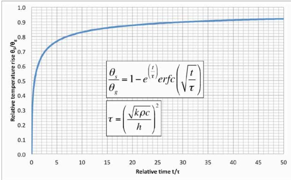
Figure 16 Laplace solution for heat transfer to semi-infinite solids.
