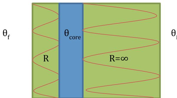
Figure 18 Thermally thin core that is completely insulated on the non-fire exposed side, a constant thermal resistant  $R$  on the fire-exposed side and a constant fire temperature  $\theta_f$ .
