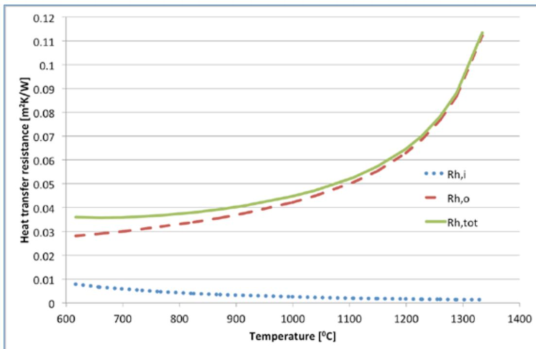
Figure 25 Convection- and radiation heat transfer resistance for the fire exposed side and the non-fire exposed side at steady state conditions for different maximal fire temperature caused by higher amount of insulation.
