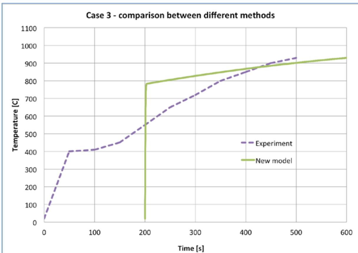
Figure 34 Comparison between different calculation methods for a steel container with insulation (case 3).
