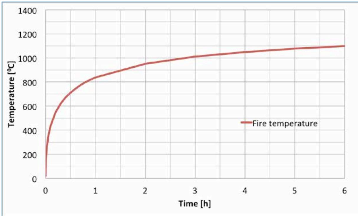
Figure 17 Calculated fire temperature for semi-infinite walls with constant parameters.  $O = 0.04 \text{ m}^{1/2}$ ,  $c_p = 1150 \text{ J/kgK}$ ,  $\alpha_1 = 0.5 \text{ kg}_{\text{air}}/\text{m}^{5/2}\text{s}$ ,  $\alpha_2 = 1518000$ ,  $\sqrt{k\rho c} = 1160 \text{ W s}^{1/2}/\text{m}^2\text{K}$ .
