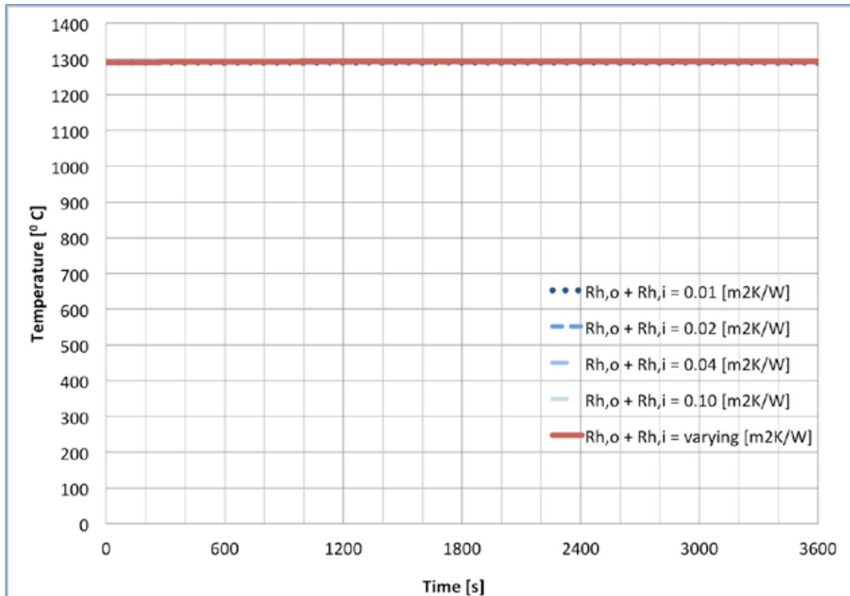
Figure 30 Fire temperature with constant- and varying convection and radiation heat transfer resistances.  $R_{ins,i} = 1.1 \text{ m}^2\text{K/W}$  and  $R_{ins,o} = 0 \text{ m}^2\text{K/W}$ .  $R_{h,i}$  and  $R_{h,o}$  are varying as in equation (67) and (68).
