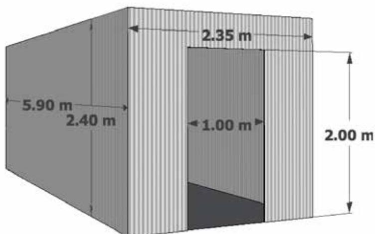
Figure 31 Compartment geometry used in case 1,2 and 3 (Back 2012).
