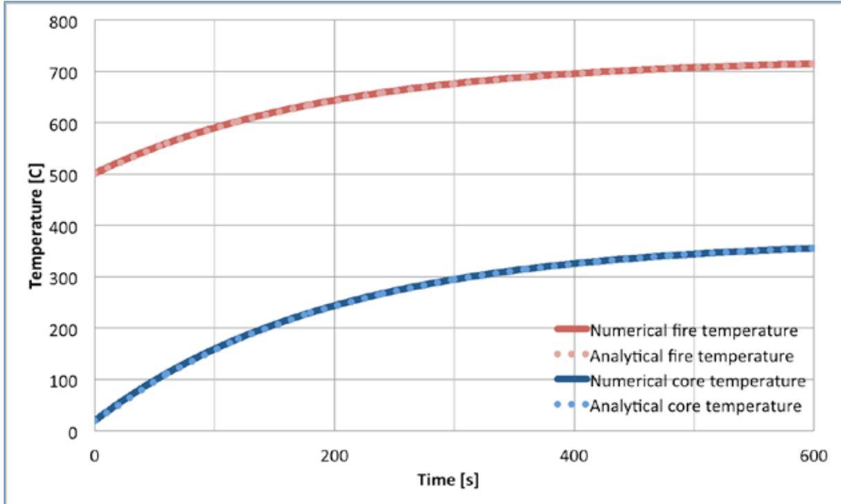
Figure 20 Calculated fire- and core temperatures by analytical and numerical solutions with the same parameters.
