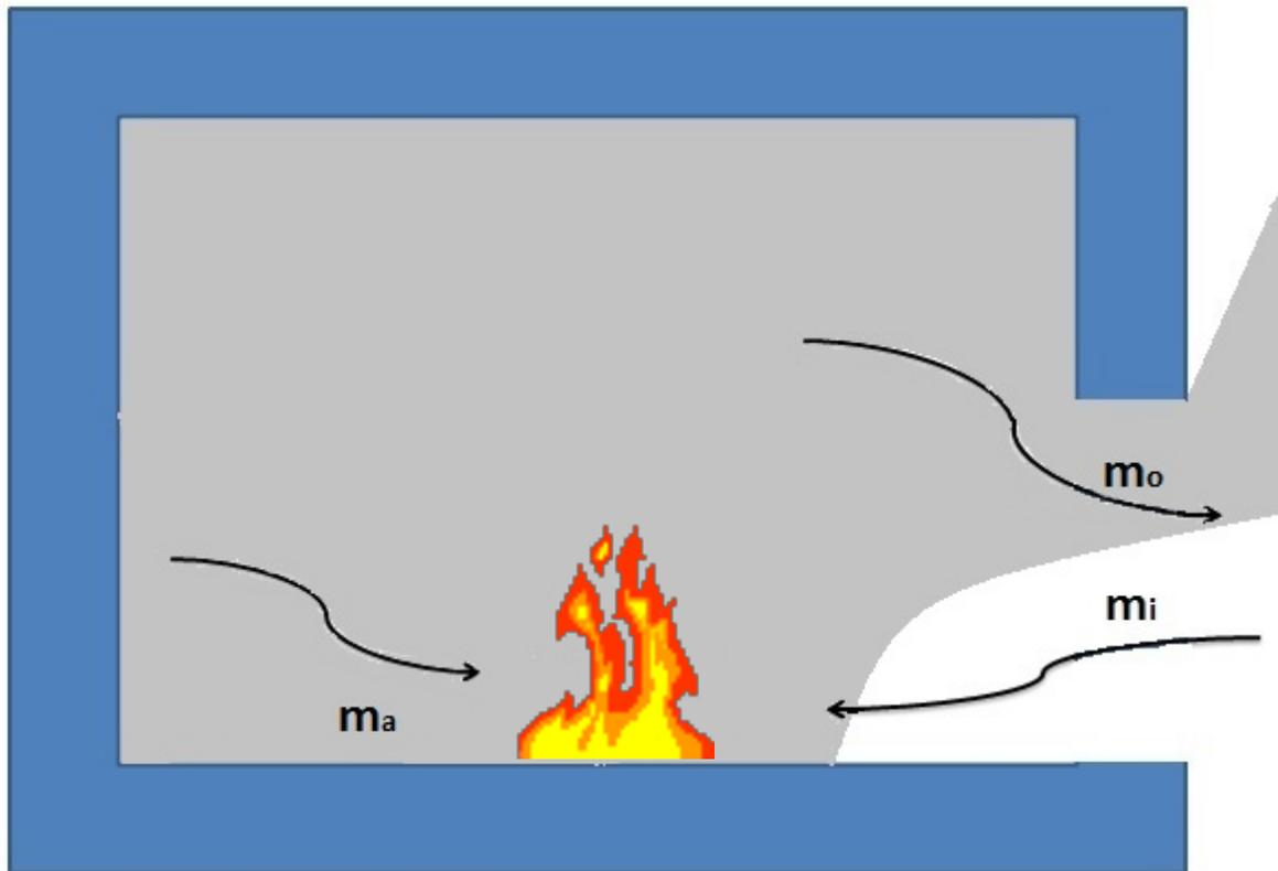
Figure 3 Mass flow for the one-zone model.
