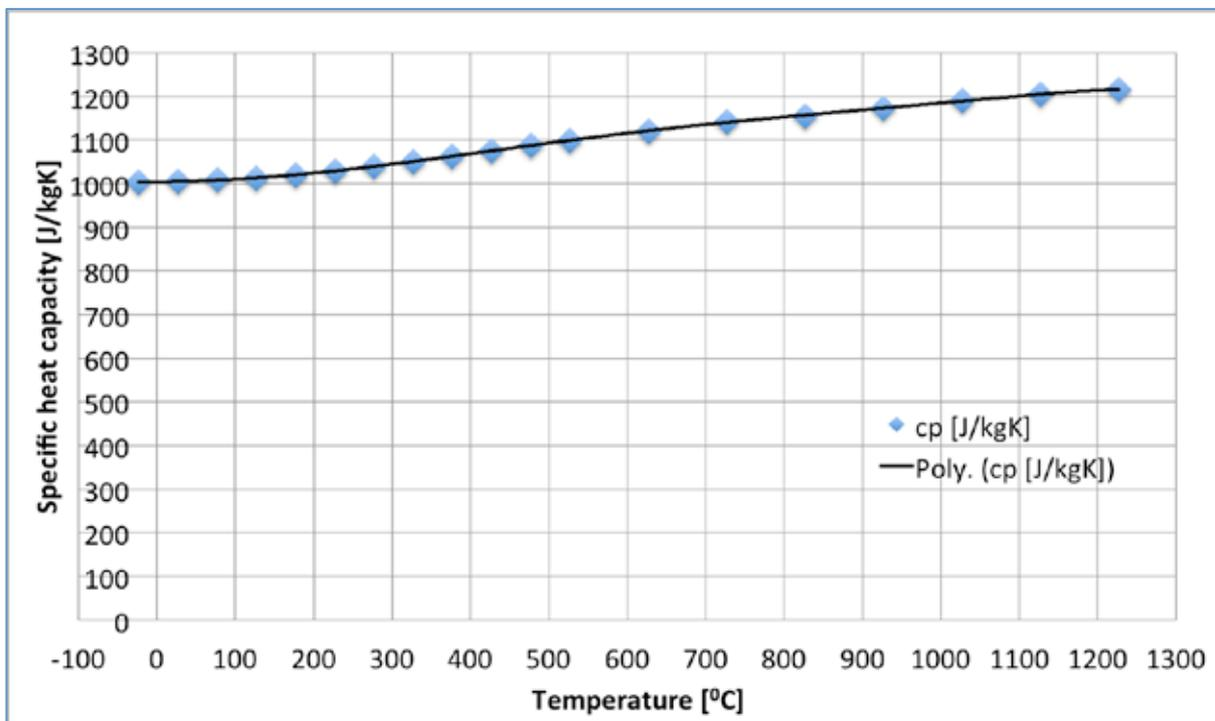
Figure 22 Specific heat capacity for air depending on temperature (Society of Fire Protection Engineers 2002) and a 6<sup>th</sup> order polynomial trend line.
