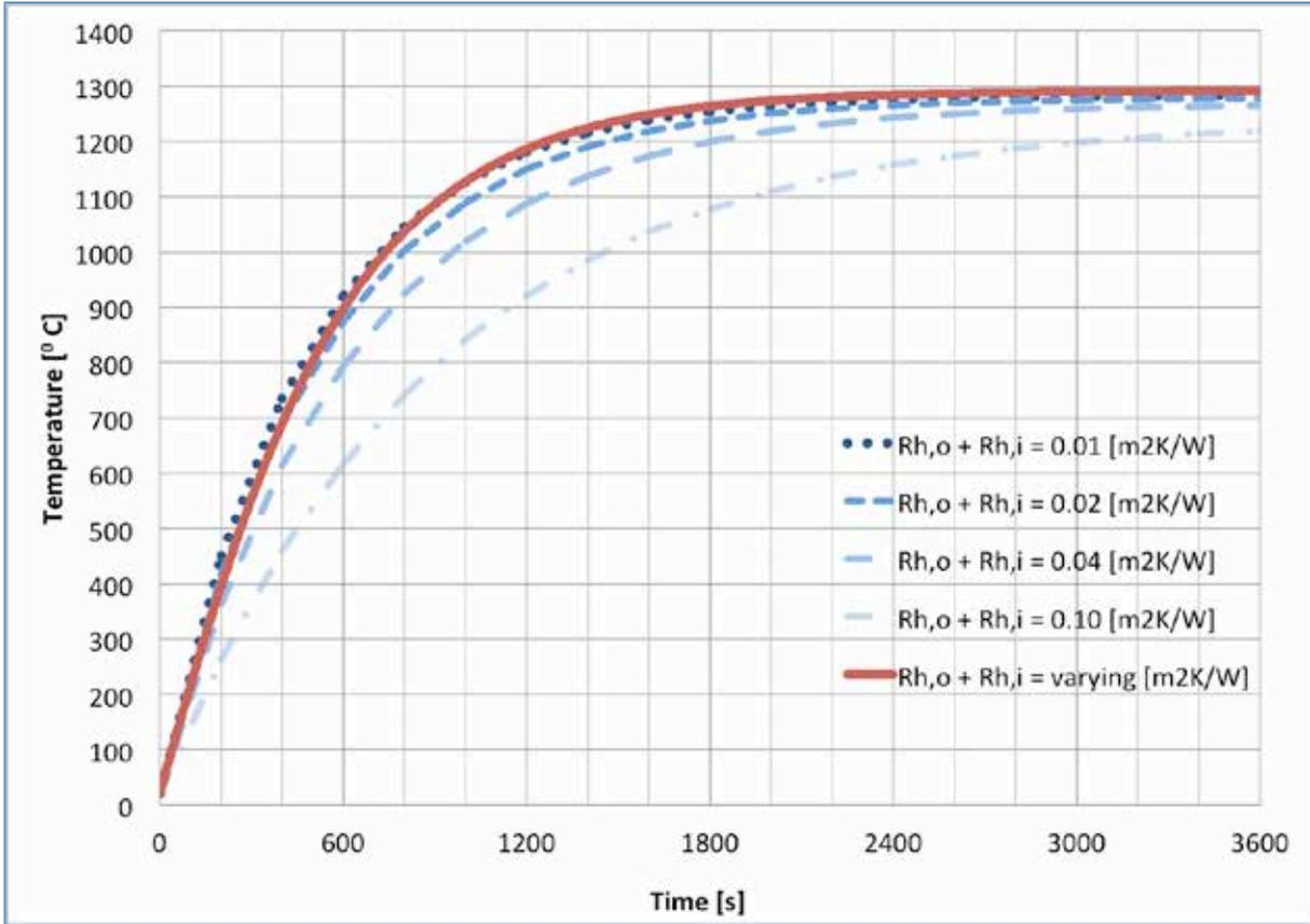
Figure 29 Core temperature with constant- and varying convection and radiation heat transfer resistances.  $R_{ins,i} = 0 \text{ m}^2\text{K/W}$  and  $R_{ins,o} = 1.1 \text{ m}^2\text{K/W}$ .  $R_{h,i}$  and  $R_{h,o}$  are varying as in equation (67) and (68).
