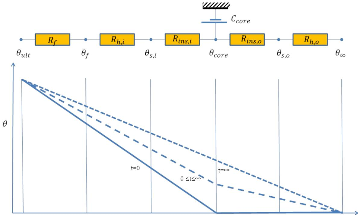
Figure 21 Schematic temperature distribution inside a thermally thin surrounding structure assuming lumped heat and an indication of the temperature in the beginning ( $t=0$ ), after some time ( $0 \leq t \leq \infty$ ) and after very long time ( $t=\infty$ ).
