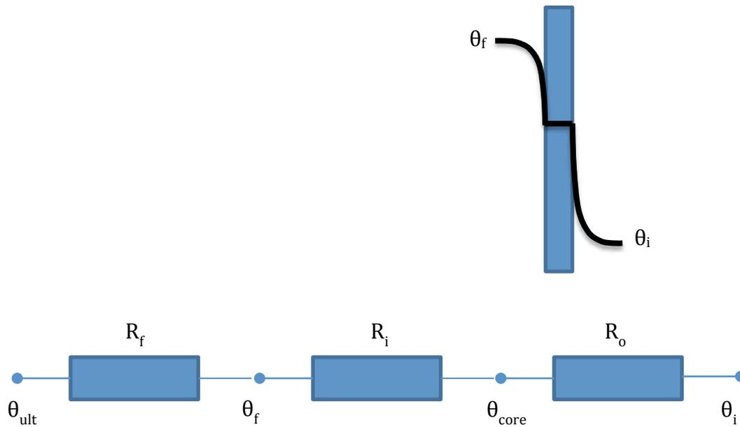
Figure 11 Temperature distribution within a thermally thin surrounding structure without insulation. The series below shows an electrical analogy with the resistances, heat capacity and the temperatures across the surrounding structures.
