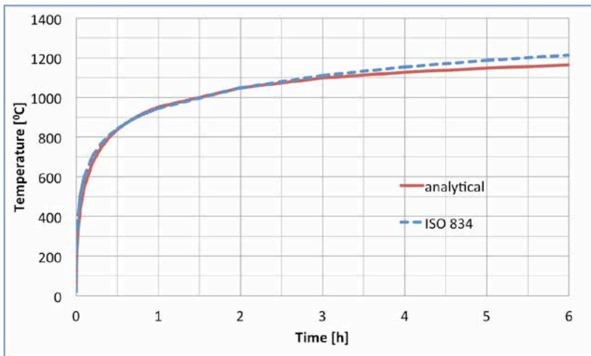
Figure 24 Calculated fire temperatures for semi-infinite walls with constant parameters.  $O = 0.04 \text{ m}^{1/2}$ ,  $c_p = 1150 \text{ J/kgK}$ ,  $\alpha_1 = 0.5 \text{ kg}_{\text{air}}/\text{m}^{5/2}\text{s}$ ,  $\alpha_2 = 1518000 \text{ J/kg}$ ,  $\sqrt{k\rho c} = 1160 \text{ W s}^{1/2}/\text{m}^2\text{K}$  and  $\tau = 1270 \text{ s}$ .
