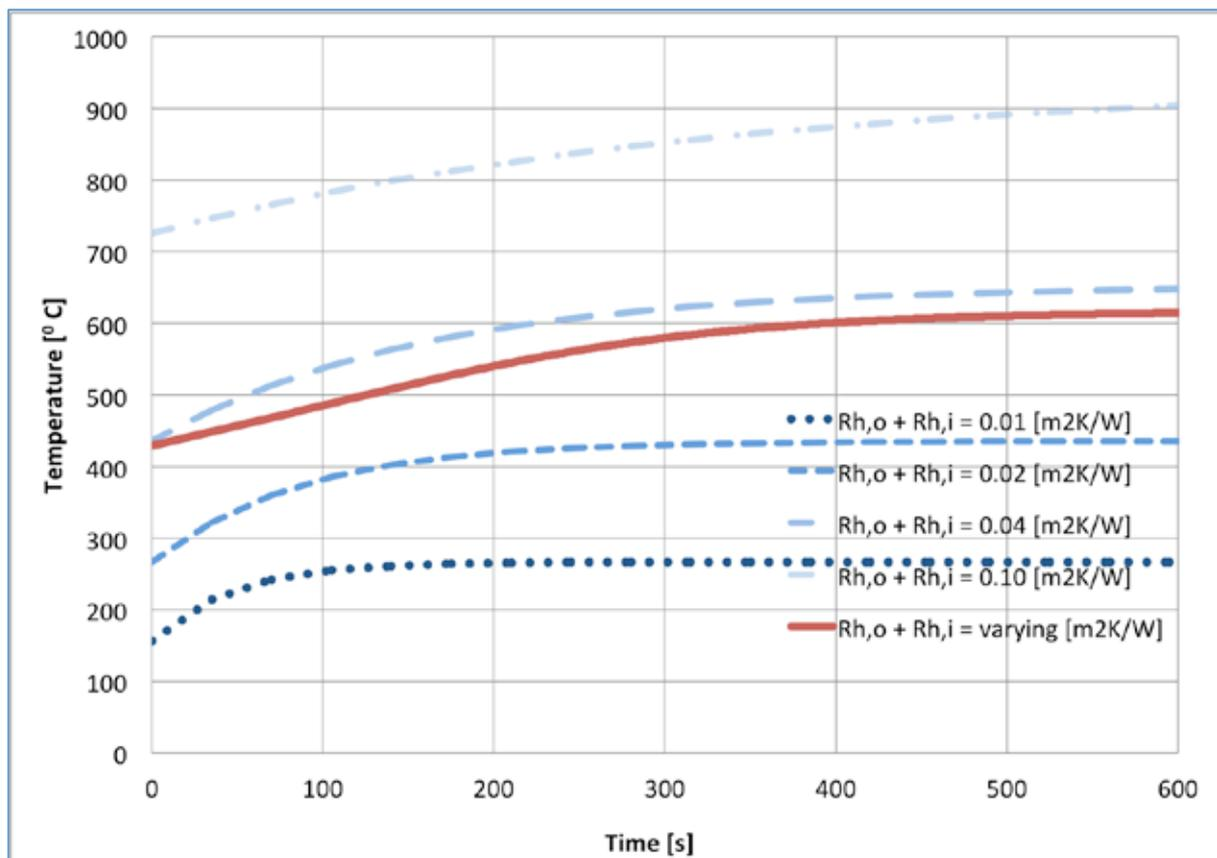
Figure 27 Fire temperature with constant- and varying convection and radiation heat transfer resistances.  $R_{ins,i} = R_{ins,o} = 0$  m<sup>2</sup>K/W.  $R_{h,i}$  and  $R_{h,o}$  are varying as in equation (67) and (68).
