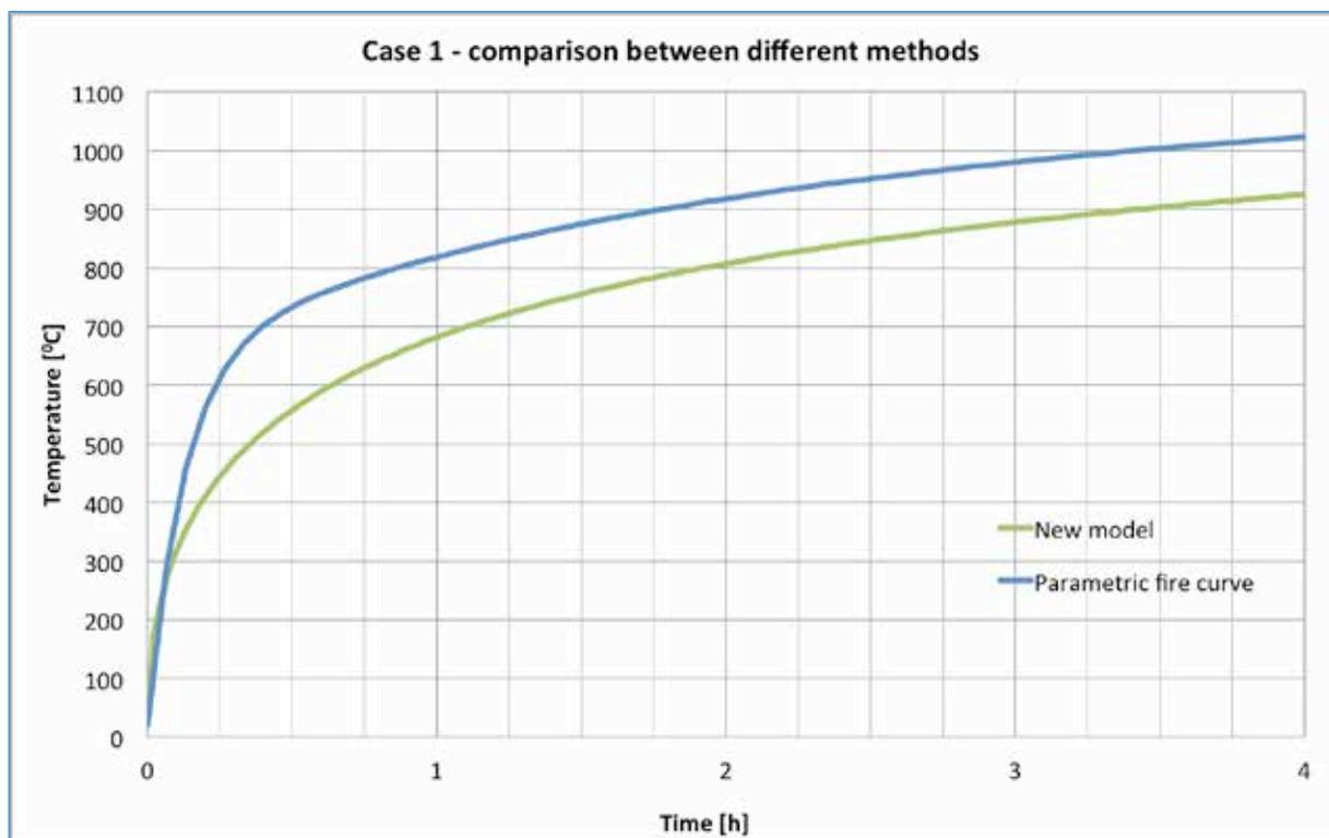
Figure 32 Comparison between different calculation methods for a concrete bunker (case 1).
