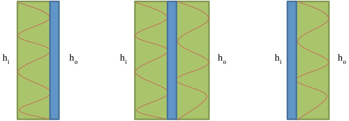
Figure 14 Thin solids with insulation on the fire-exposed side, on the non-fire exposed side and on both sides.  $h_i$  [W/m<sup>2</sup>K] is the heat transfer coefficient on the fire exposed side and  $h_o$  [W/m<sup>2</sup>K] is the heat transfer coefficient on the non-fire exposed side.
