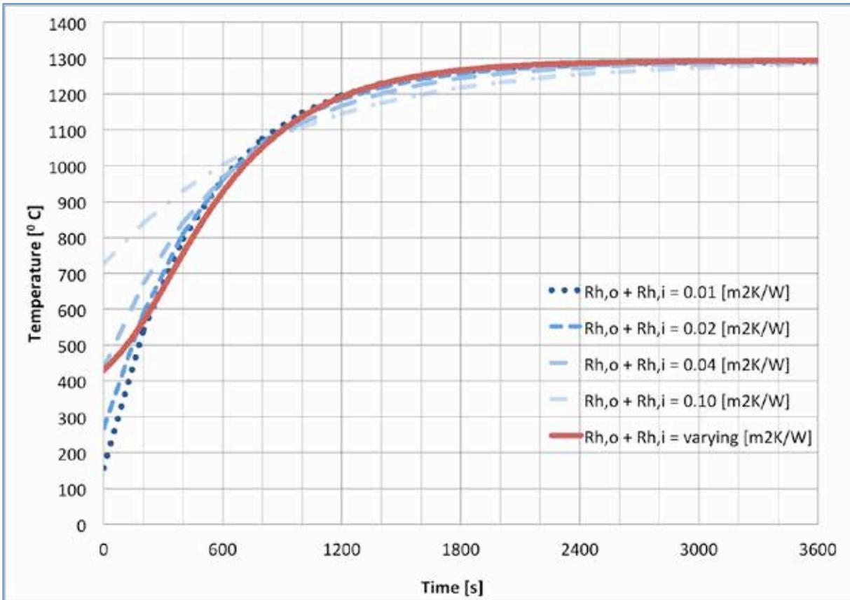
Figure 28 Fire temperature with constant- and varying convection and radiation heat transfer resistances.  $R_{ins,i} = 0 \text{ m}^2\text{K/W}$  and  $R_{ins,o} = 1.1 \text{ m}^2\text{K/W}$ .  $R_{h,i}$  and  $R_{h,o}$  are varying as in equation (67) and (68).
