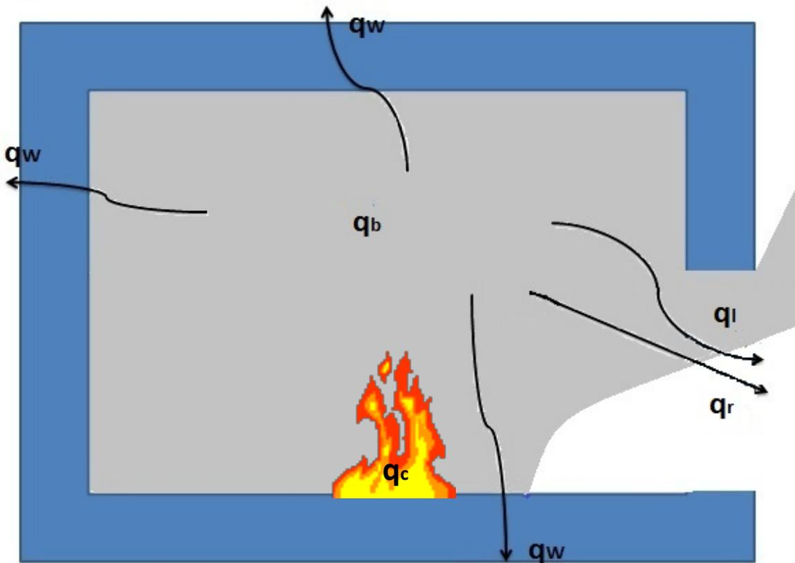
Figure 2 Energy balance illustrated for one-zone model.
