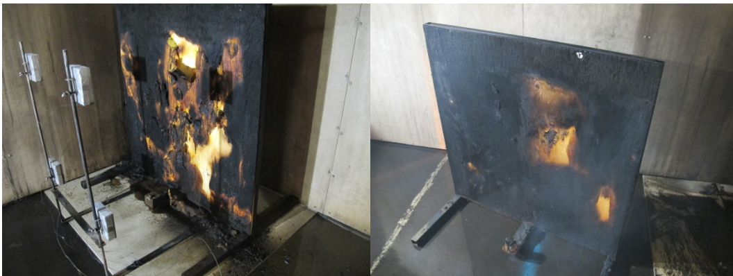
Figure 32 Fire damages: The stand-alone water mist system flowing 8.2 liter/min at 120 bar, when ignition was at the front (left) or back of the simulated upholstered chair (right).
