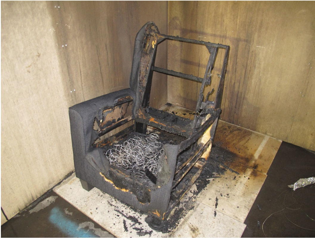
Figure 34 Fire damages: Residential sprinkler having a 3 mm, 68°C glass bulb flowing 30.3 liter/min.
