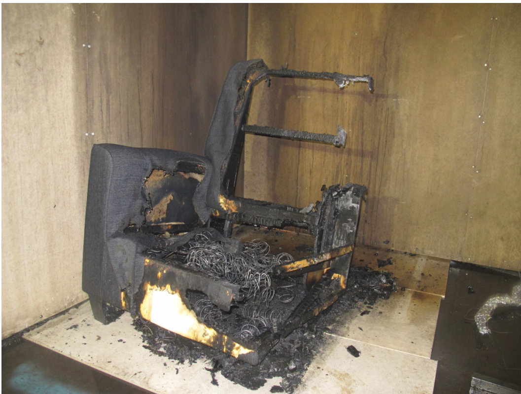
Figure 35 Fire damages: Residential sprinkler having a 3 mm, 57°C glass bulb flowing 30.3 liter/min.
