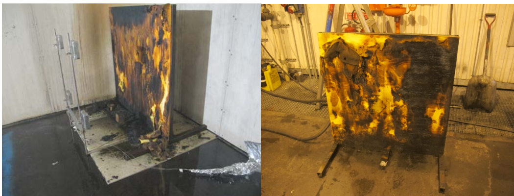
Figure 29 Fire damages: The multi-orifice low-pressure water mist nozzle flowing 32 liter/min at 5.2 bar, when ignition was at the front (left) or back of the simulated upholstered chair (right).
