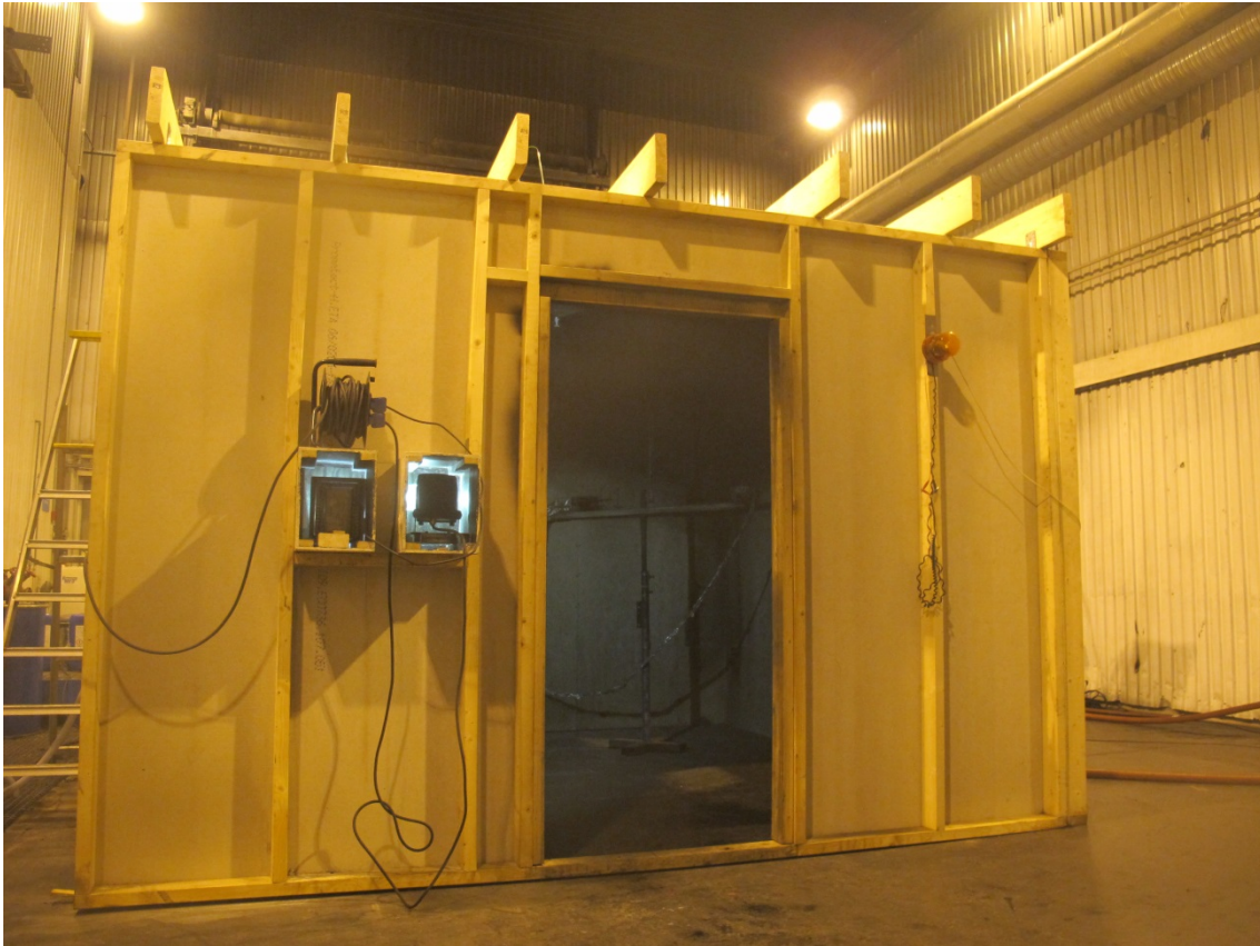
Figure 1 The fire test compartment used in the tests. The compartment was sized 3.66 m by 3.66 m and had a regular doorway opening at centerline of the front wall.
