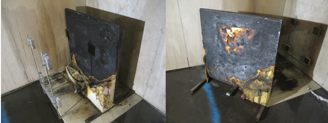
Figure 30 Fire damages: The multi-orifice high-pressure water mist nozzle flowing 17.2 liter/min at 52 bar, when ignition was at the front (left) or back of the simulated upholstered chair (right).
