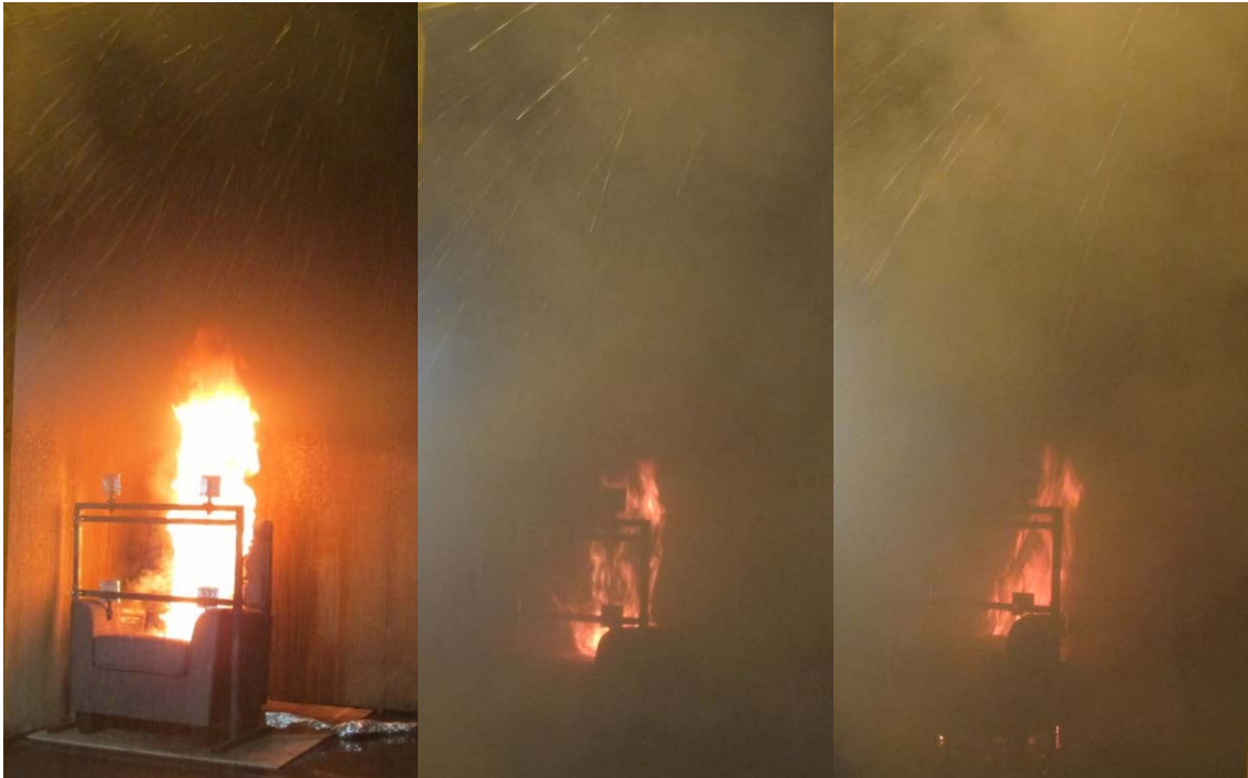
Figure 12 Fire events: Residential sprinkler having a 3 mm, 68°C glass bulb flowing 60.6 liter/min, at 1) moments after the activation at 68 seconds, 2) one minute after activation and 3) two minutes after activation.
