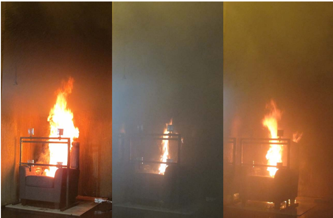
Figure 13 Fire events: The single-orifice low-pressure water mist nozzle flowing 23.4 liter/minute at 7.6 bar, at 1) moments prior the activation at 60 seconds, 2) one minute after activation and 3) two minutes after activation.
