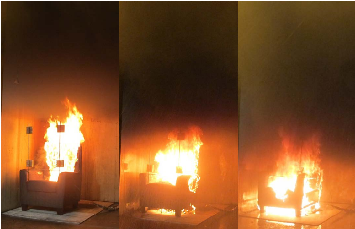
Figure 9 Fire events: Residential sprinkler having a 3 mm, 68°C glass bulb flowing 30.3 liter/min, at 1) moments prior the activation at 60 seconds, 2) one minute after activation and 3) two minutes after activation.
