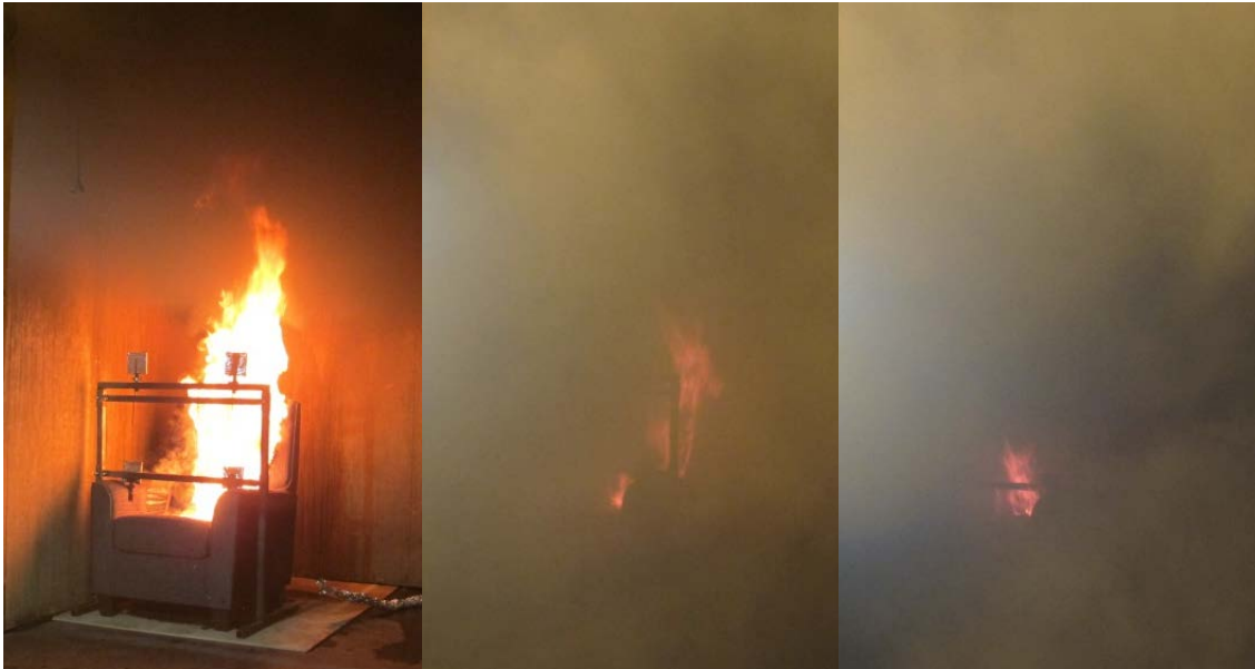
Figure 14 Fire events: The multi-orifice low-pressure water mist nozzle flowing 32 liter/min at 5.2 bar, at 1) moments prior the activation at 66 seconds, 2) one minute after activation and 3) two minutes after activation.
