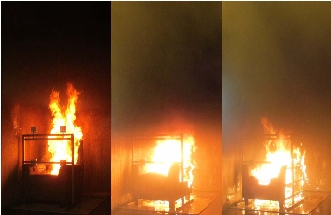
Figure 10 Fire events: Residential sprinkler having a 3 mm, 57°C glass bulb flowing 30.3 liter/min, at at 1) moments after the activation at 55 seconds, 2) one minute after activation and 3) two minutes after activation.
