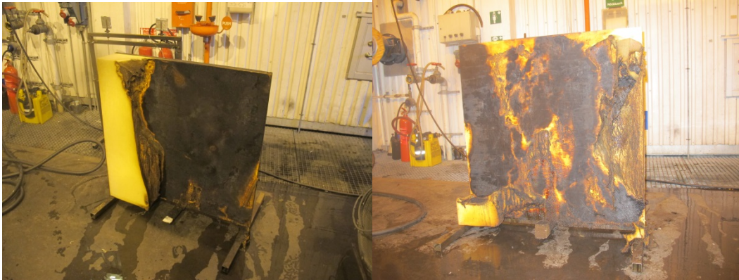
Figure 27 Fire damages: Residential sprinkler having a 3 mm, 68°C glass bulb flowing 60.6 liter/min, when ignition was at the front (left) or back of the simulated upholstered chair (right).
