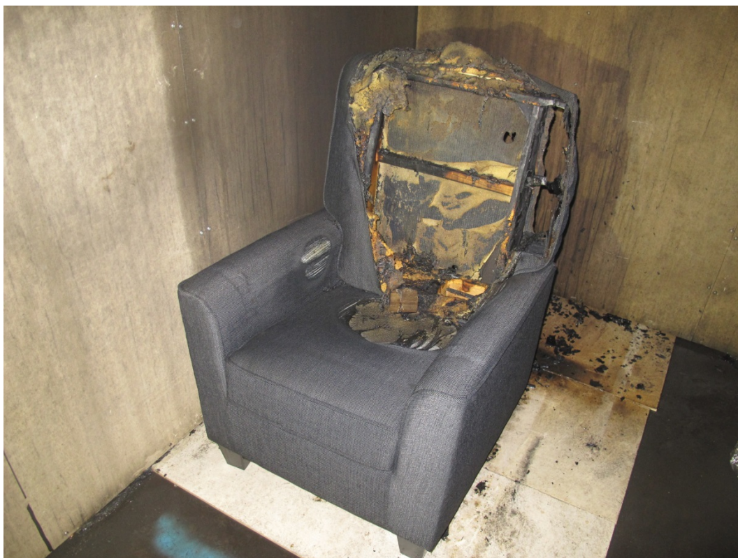
Figure 40 Fire damages: The multi-orifice high-pressure nozzle flowing 36.7 liter/min at 80 bar.
