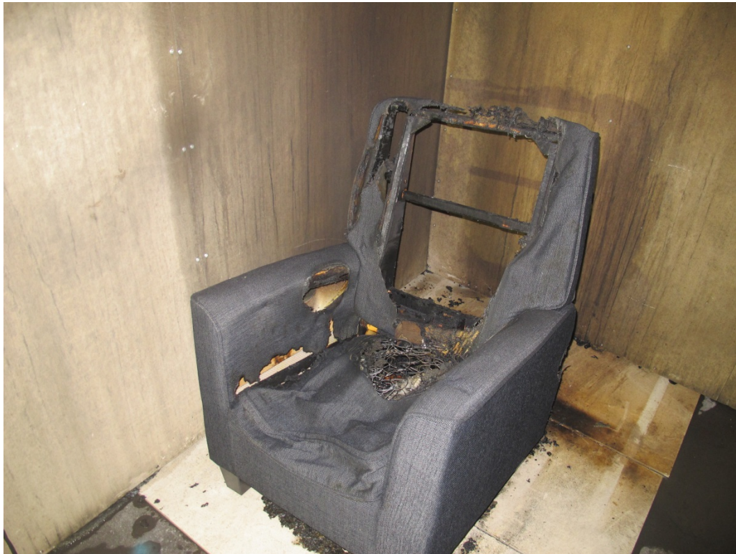
Figure 38 Fire damages: The single-orifice low-pressure water mist nozzle flowing 23.4 liter/minute at 7.6 bar.
