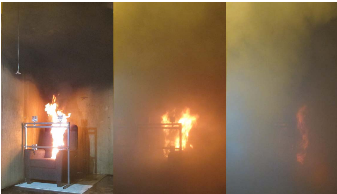
Figure 17 Fire events: The stand-alone water mist system flowing 8.2 liter/min at 120 bar, at 1) moments prior the activation at 43 seconds, 2) one minute after activation and 3) two minutes after activation.
