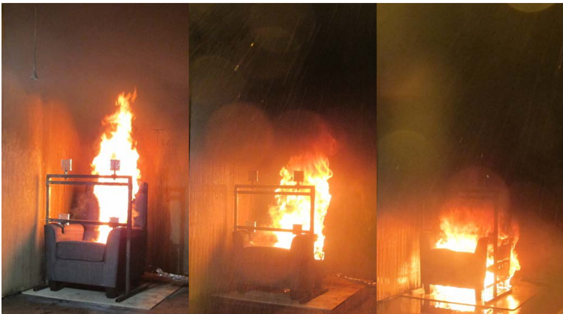
Figure 11 Fire events: Residential sprinkler having a 2.5 mm, 47°C glass bulb flowing 30.3 liter/min, at 1) moments prior the activation at 51 seconds, 2) one minute after activation and 3) two minutes after activation.
