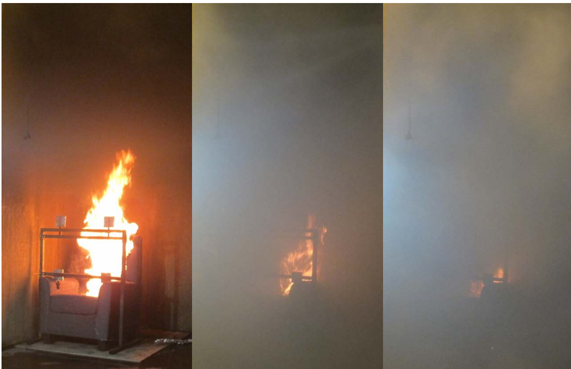
Figure 15 Fire events: The multi-orifice high-pressure nozzle flowing 36.7 liter/min at 80 bar, at 1) moments prior the activation at 64 seconds, 2) one minute after activation and 3) two minutes after activation.
