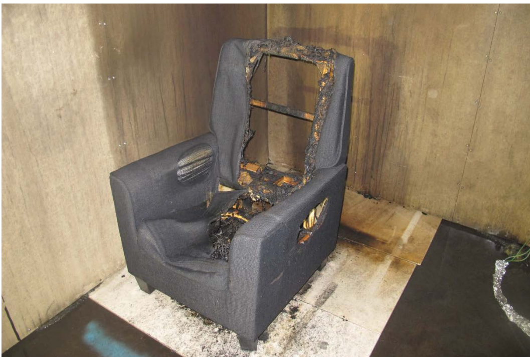
Figure 37 Fire damages: Residential sprinkler having a 3 mm, 68°C glass bulb flowing 60.6 liter/min.
