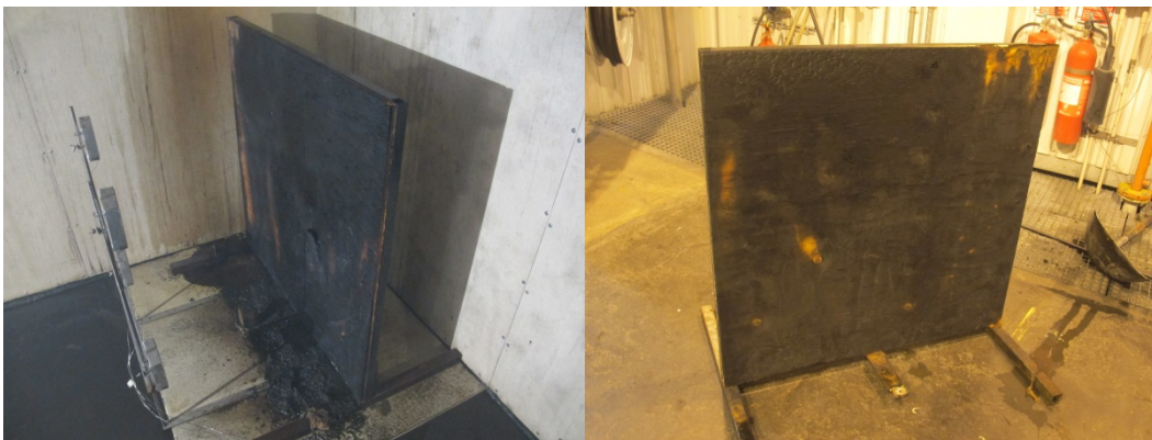
Figure 28 Fire damages: The single-orifice low-pressure water mist nozzle flowing 23.4 liter/minute at 7.6 bar, when ignition was at the front (left) or back of the simulated upholstered chair (right).
