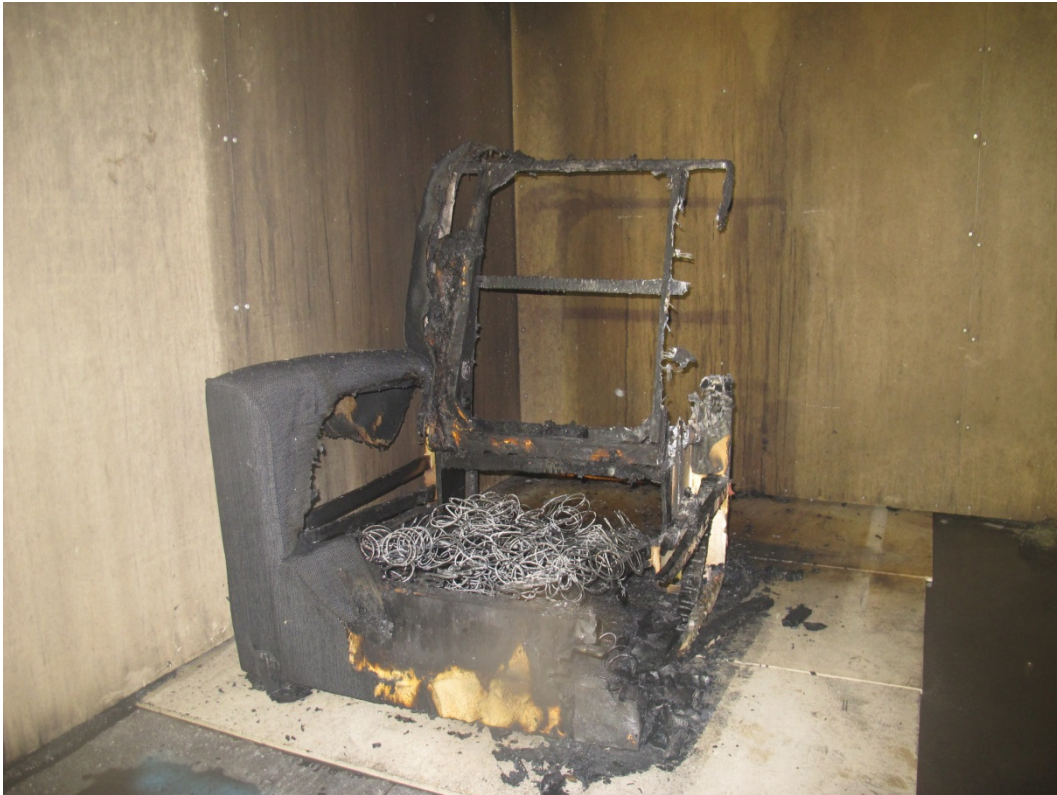
Figure 36 Fire damages: Residential sprinkler having a 2.5 mm, 47°C glass bulb flowing 30.3 liter/min.
