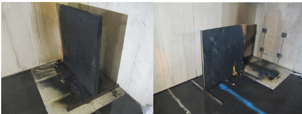
Figure 26 Fire damages: Residential sprinkler having a 3 mm, 68°C glass bulb flowing 30.3 liter/min, when ignition was at the front (left) or back of the simulated upholstered chair (right). Note: For all other residential sprinkler tests at 30.3 liter/min the fire damages were similar and these photos are therefore not included.
