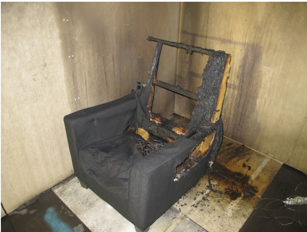
Figure 42 Fire damages: The stand-alone water mist system flowing 8.2 liter/min at 120 bar.
