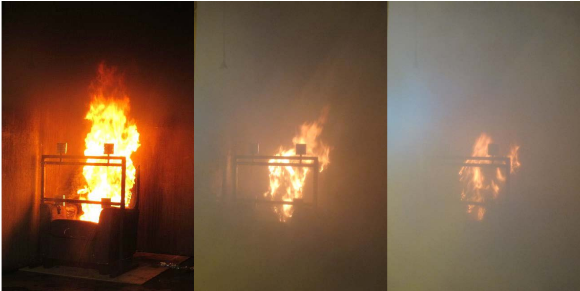
Figure 16 Fire events: The multi-orifice high-pressure water mist nozzle flowing 17.2 liter/min at 52 bar, at 1) moments prior the activation at 70 seconds, 2) one minute after activation and 3) two minutes after activation.
