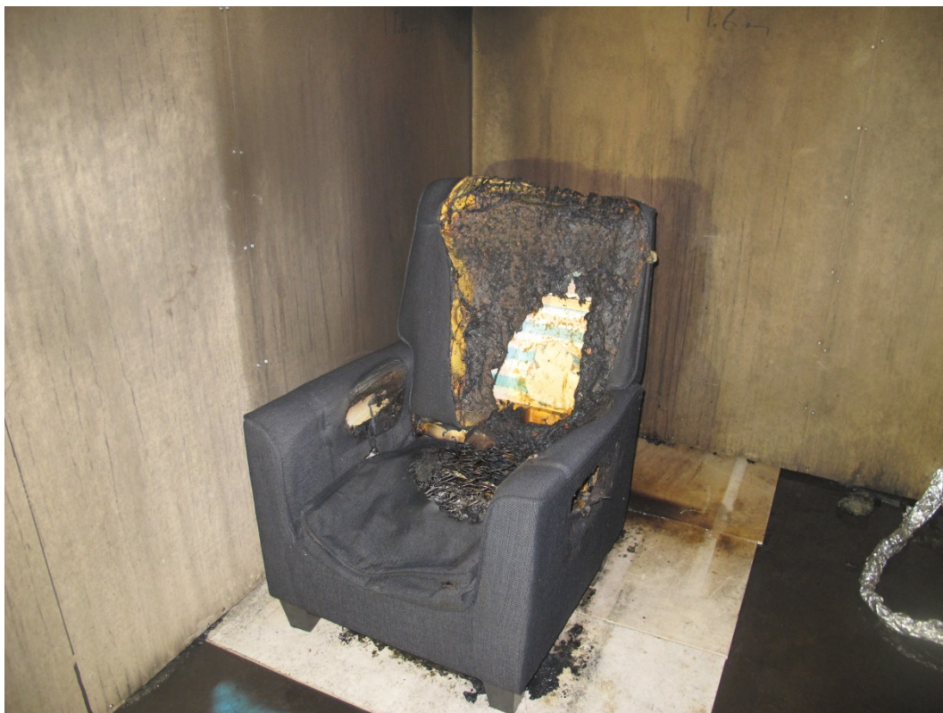
Figure 39 Fire damages: The multi-orifice low-pressure water mist nozzle flowing 32 liter/min at 5.2 bar.
