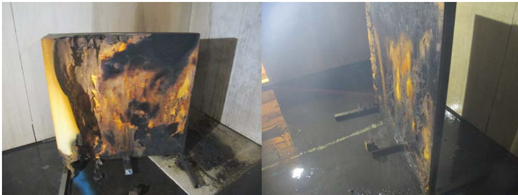
Figure 31 Fire damages: The multi-orifice high-pressure nozzle flowing 36.7 liter/min at 80 bar, when ignition was at the front (left) or back of the simulated upholstered chair (right).
